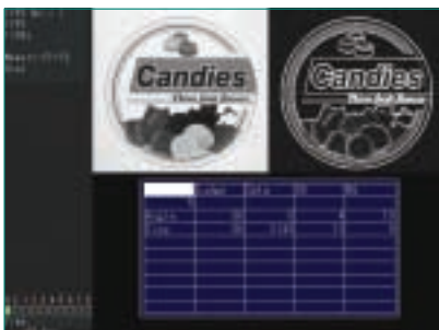
Simultaneous image display from two cameras (This shows an image processed with gray scale and binary differentiation.)
